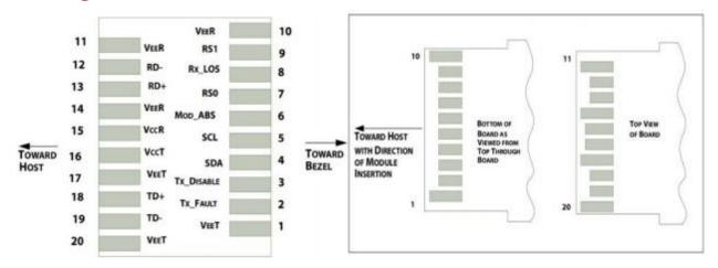
Host PCB SFP+ pad assignment top view and Names.
