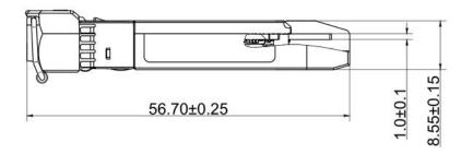
Unit:mm Unspecified Tolerance:±0.1mm
